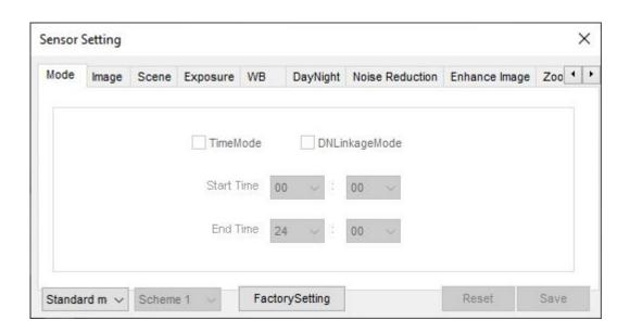
In order to change these settings you must first change the mode in the lower left, from Standard Mode to Debug mode as in the figure below. The debug mode allows you to modify the sensor parameters and then save and return to the Standard operating mode.
