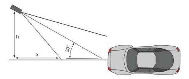
The minimum reading distance X depends on the positioning height of the camera according to the formula X = Hx1.7. For example, if the camera is positioned at 3 meters, the minimum reading distance is 5.1 m.
