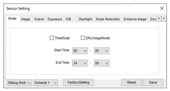
The debug mode allows you to set up to 4 customized configurations (DIAGRAM 1,2,3,4) to be activated according to the situation. These license plate cameras use the first 2 configurations: SCHEMA1 during the day and SCHEMA2 at night which are already configured at the factory for an optimal recovery in the two situations.
